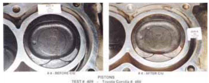
Picture G - Piston before P.i. treatment
