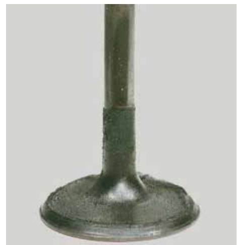
Picture E - Intake valve after P.i. treatment
